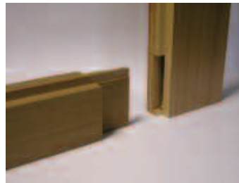
Mortice and tenon joint
